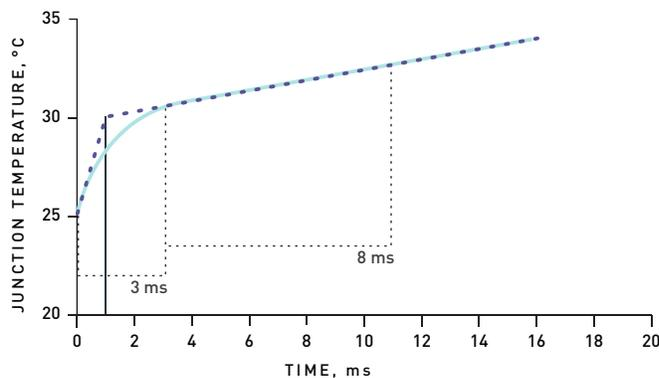
Crystal IS measures Klaran device power by waiting 3 ms after the start of the current pulse and then integrate the output for 8 ms.
