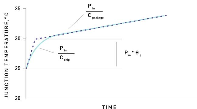
A very simple model for the rise in junction temperature for a typical Crystal IS Klaran diode after power is applied to the device.
