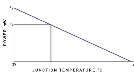
*Illustration of how a design engineer can determine the tradeoff of maintaining junction temperature to achieve required UVC output power.*
