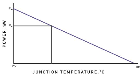
*Illustration of how a design engineer can determine the tradeoff of maintaining junction temperature to achieve required UVC output power.*
