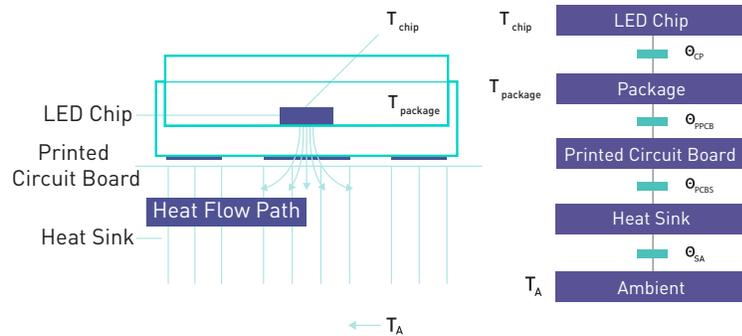
A simplified illustration indicating the Chip Temperature ( $T_{chip}$ ), Package Temperature ( $T_{package}$ ) and Ambient Temperature ( $T_A$ ).
