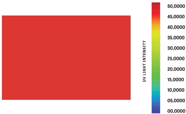
FIGURE 4B: Irradiance model of Duct 2 lined with 80% UV reflective materials on all four sides.
